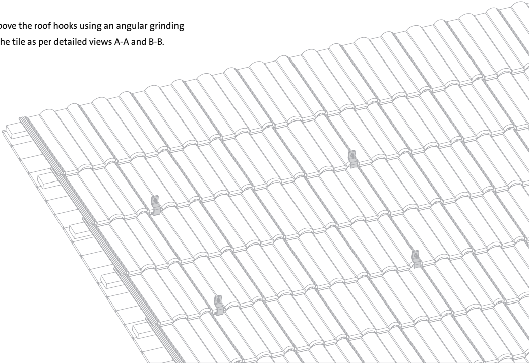
One-layer rail system on tongue and groove boards fixation - vertical module alignment
