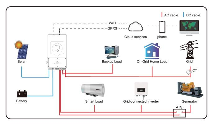
The hybrid inverter will not only provide power to the backup load connected but also give power to the home load connected. If PV power and battery power are insufficient, it will take grid energy as a supplement. The hybrid inverter will not sell power to the grid. The external CT (&Meter) will detect power flowing back to the grid and will reduce the power of the inverter only to supply the local load and charge the battery and home load. This control is achieved by:
